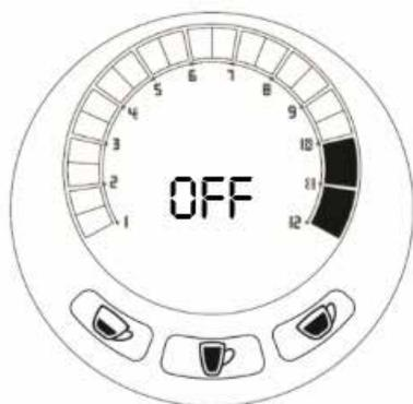
To turn the group on again, press buttons (B) and (C) together.
