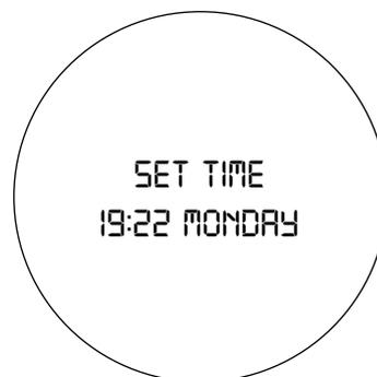
The modifiable value flashes. To change the value, press buttons (A) or (C), then press button (B) to confirm the choice and move on to the next value to be set.
