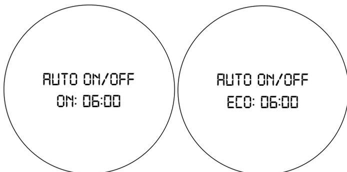
To change the values, press buttons (A) or (C), then press button (B) to confirm the choice and move on to the next values to be set .
